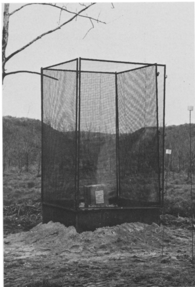
Fig. 1. Fire cage before the test with 25 kg of t-butyl perbenzoate.
