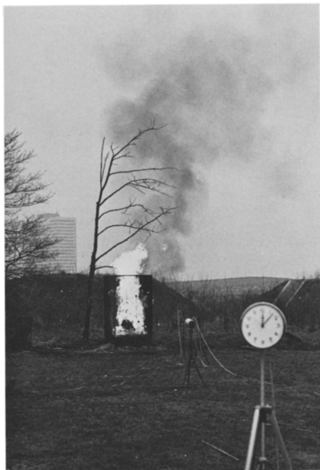
Fig. 3. Typical photograph of a fire of 100 kg of cyclohexanone peroxide at its height.
