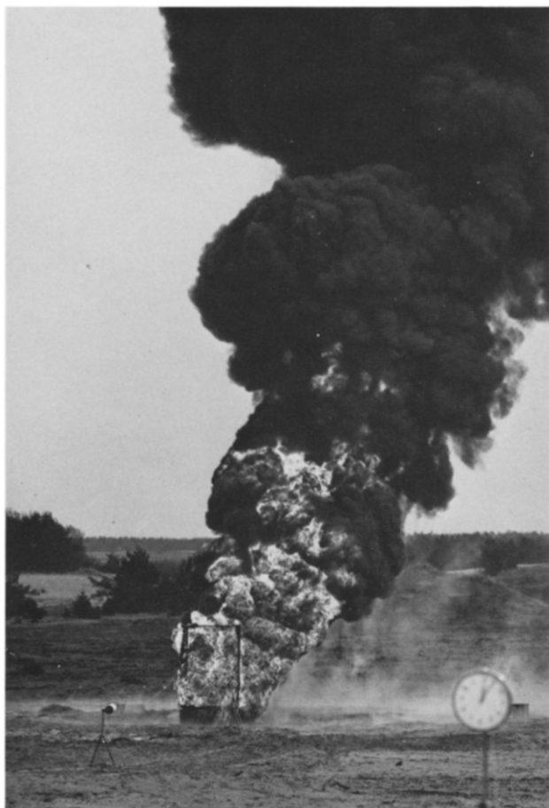
Fig. 4. Typical photograph of a fire of 500 kg of t-butyl perbenzoate.
